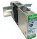
RPM(D)    | 15-60     | 9.5-18, 9.5-36, 10-40, (D)<br>18-36, 18-75, 36-75 | 3.3, 5, 12, 15, ±5, ±12, ±15<br>5/±12, 5/±15 | 1.6 kVDC / 1 min  | 101.6 x 57.2 x 19.0 mm (4.0" x 2.3" x 0.7")<br>24.5 x 57.6 x 125.0 mm (D)<br>(1.0" x 2.3" x 4.9")  | EN/IEC60950-1                                                              | Reverse polarity protected, soft start<br>panel mount/bulkhead version RPM<br>DIN-Rail version RPMD, screw terminals<br>triple output only for 40W version available  |
