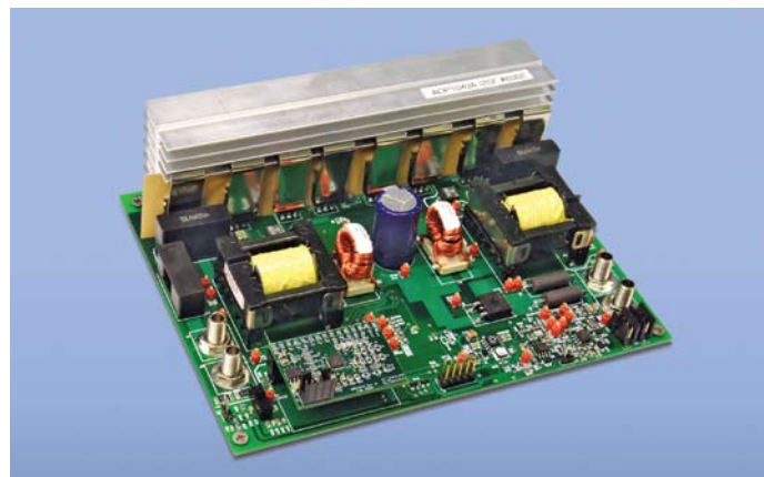
300 W interleaved 2-FET, forward evaluation design. Converts from 380 V dc to 12 V output.
